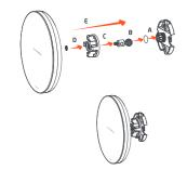
F) Thread the open end of the pole strap through the two tabs on the bracket.
